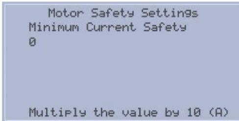
Figure 4.2 The Setting for Current Safety – Minimum Current
