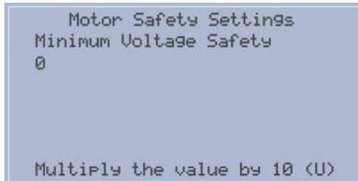
Figure 4.5 The Setting for Voltage Safety – Minimum Voltage
