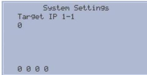
Figure 2.2 Target IP Octet 1 Setting Screen
