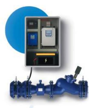
**SMART PCS** is comprised of an integrated mechanical and electronics controlling unit which is used to regulate the pressure automatically in a region. It is a novelty device developed to reduce the water losses in the water network due to the high water pressure. Depending on the consumption rates in the region, it can set the water pressure adaptively to the desired pressure value set by the user by using PID methods.
